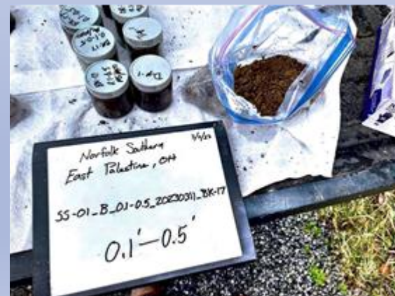
Figures 6-15 & 6-16: Arcadis's Soil Sampling Protocol – First, Place Soil Samples in Plastic Bags and then in Glass Jars (Exhibit 88, pgs. 130 and 110)
