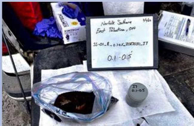
Figures 6-15 & 6-16: Arcadis's Soil Sampling Protocol – First, Place Soil Samples in Plastic Bags and then in Glass Jars (Exhibit 88, pgs. 130 and 110)
