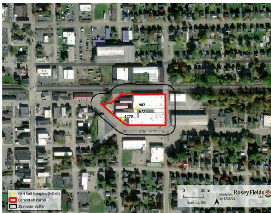
Figure 2-4. PAH Sampling at WYG Refractories Located at 193 N. James St.
