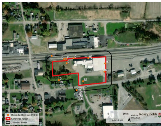
Figure 2-1. Dioxin Sampling at CeramFab Facility Located at 900 E. Taggart St.
